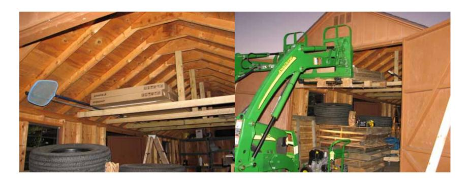
Pallet forks get the heavy load up to the correct level, then human power slides load from forks onto loft.
