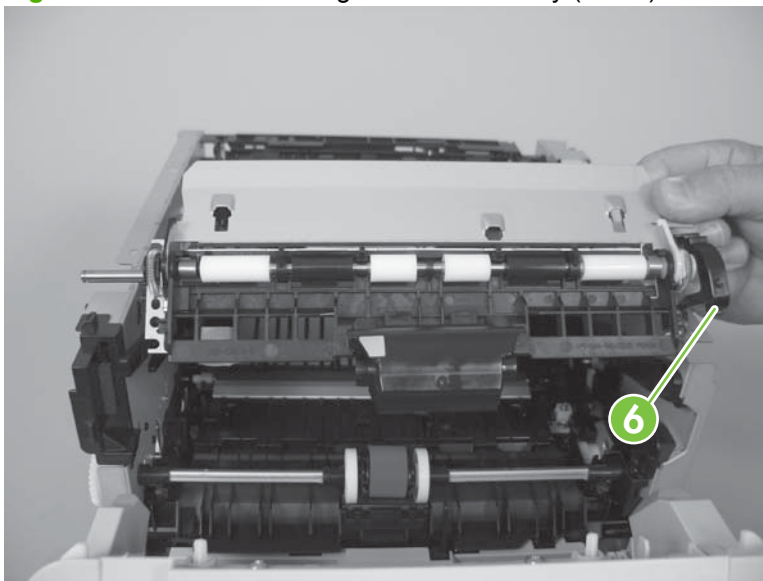
Figure 6-85 Remove the registration assembly (7 of 7)
